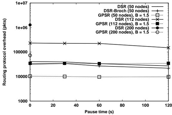
**Figure 13: Routing Protocol Overhead.** Total routing protocol packets sent network-wide during the simulation for GPSR with  $B = 1.5$  compared with DSR.  $y$  axis log-scaled. 50, 112, and 200 nodes.
