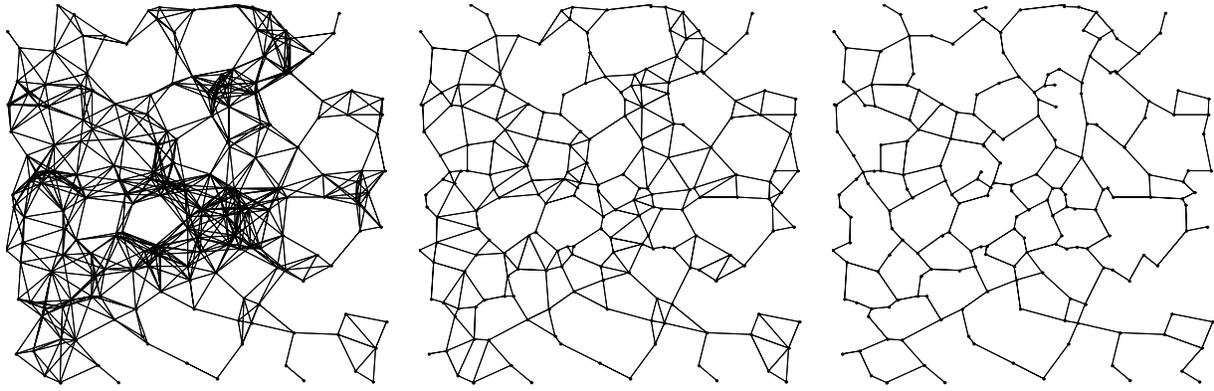
**Figure 7:** Left: the full graph of a radio network. 200 nodes, uniformly randomly placed on a 2000 x 2000 meter region, with a radio range of 250 m. Center: the GG subset of the full graph. Right: the RNG subset of the full and GG graphs.
